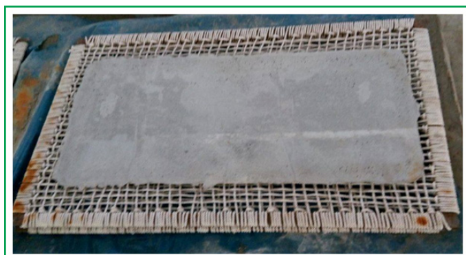
Figure 5. Completed specimen with nylon mesh
