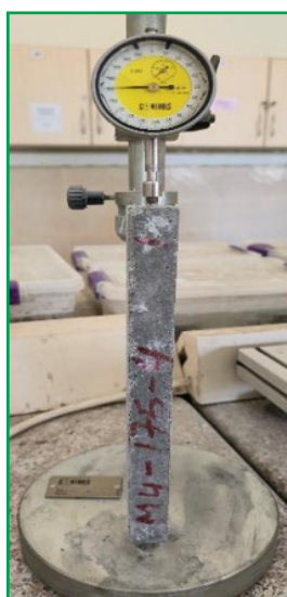
Figure 6. Drying shrinkage device for measuring the drying shrinkage of concrete
