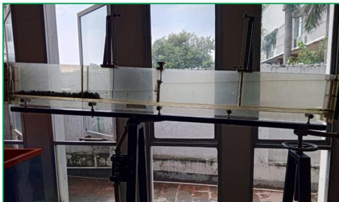
**Figure 3.** Channel at  $2.5^\circ$  adverse slope
