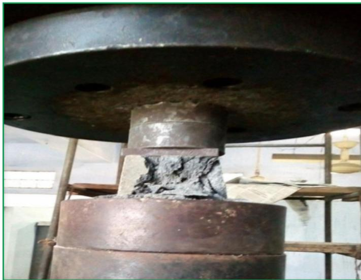
**Figure 4.** Compressive strength testing under UTM
