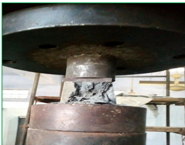
Figure 4. Compressive strength testing under UTM
