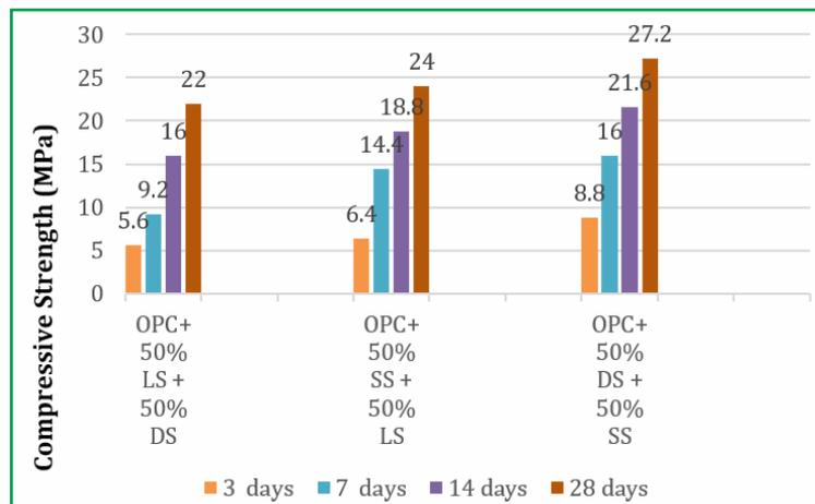
**Figure 11.** Compressive strength of cement mortar mixing multiple types of sand (1:6)
