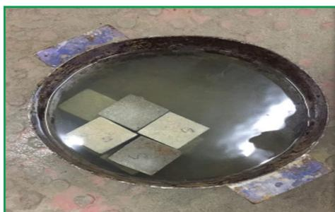
**Figure 3.** Curing of the mortar specimen
