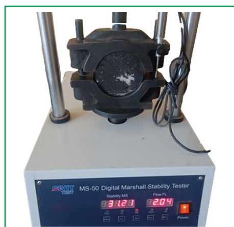
Figure 7. Marshall stability test
