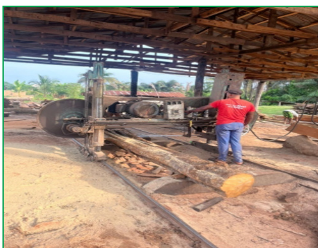
Figure 6. Cutting of the timber log into standard sizes
