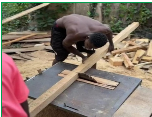
Figure 7. Cutting of the timber log into standard sizes
