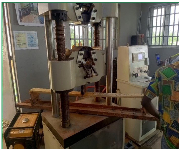
Figure 11. Laboratory setup for modulus of rupture determination
