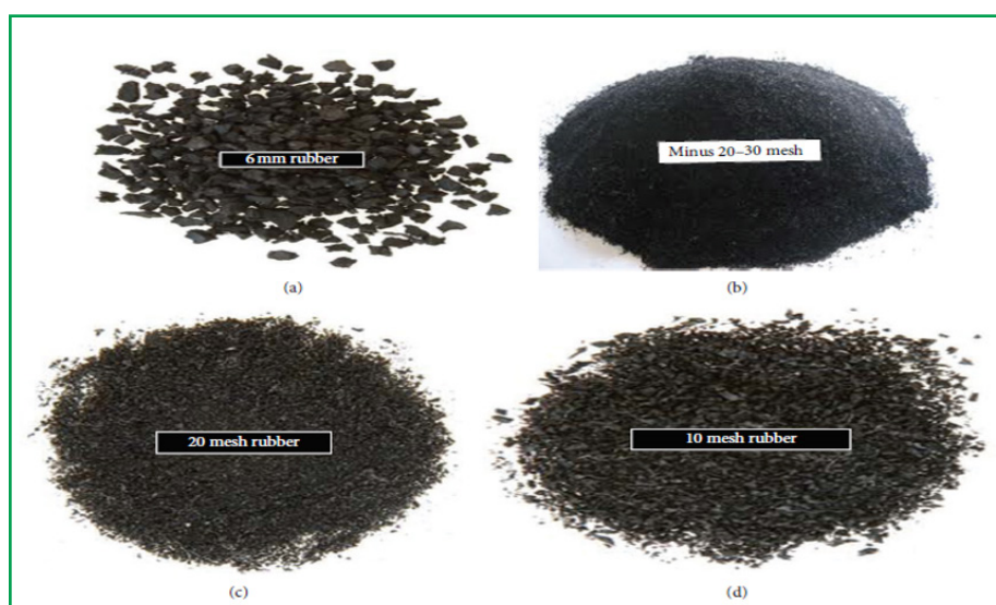
Figure 2. Different type of crumb rubber based on particle size
