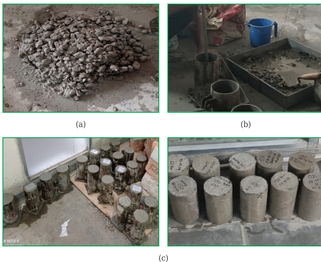
Figure 7. (a) Concrete mixing; (b) Tamping; (c) Cylinder Specimens
