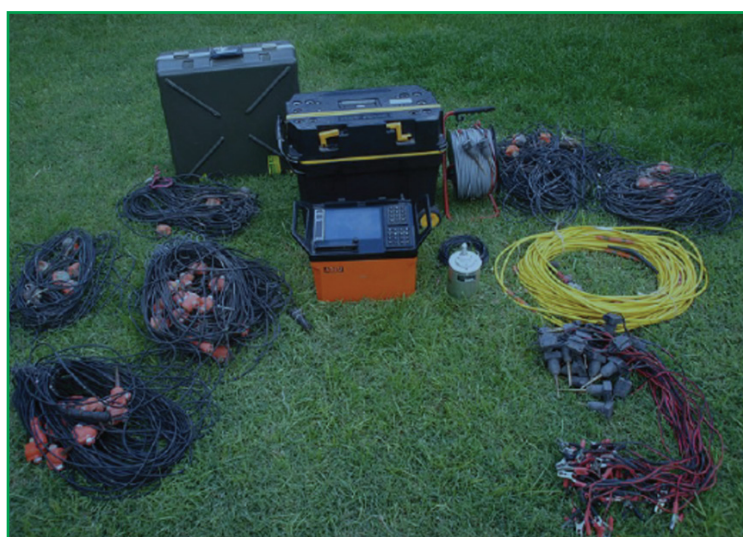
Figure 1. Seismic refraction equipment for the survey
