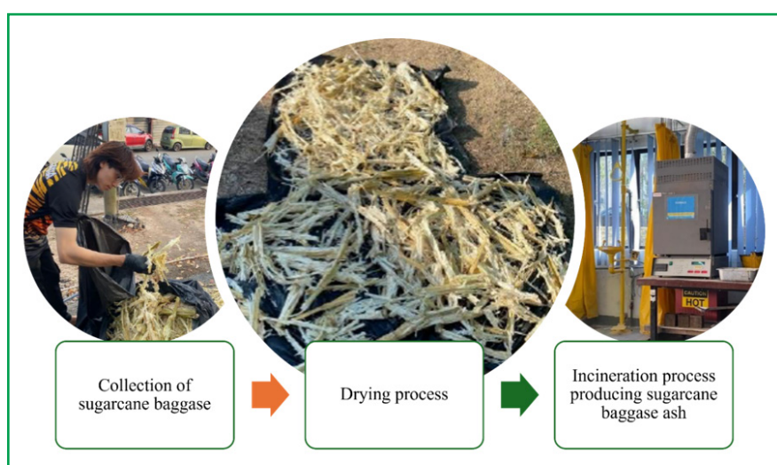
Figure 1. Preparation of sugarcane bagasse ash
