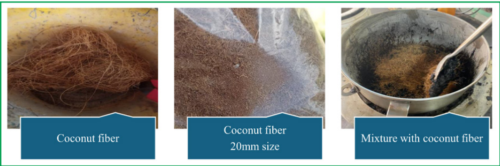
Figure 1. Preparation of coconut fiber and mixture
