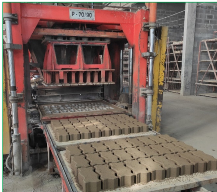
Figure 2. After demolding from machine mold
