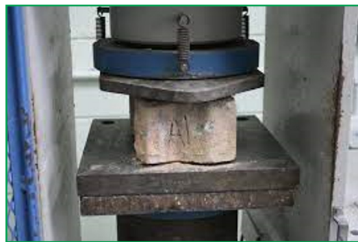
(a) compressive strength test setup
