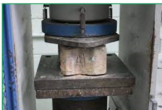
(a) compressive strength test setup
