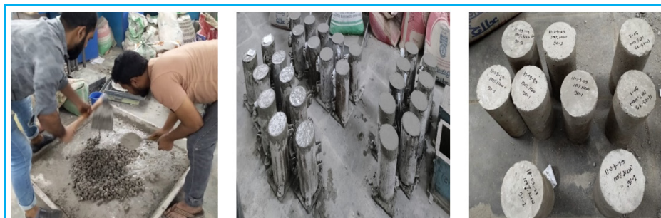
Figure 6. Casting and molding procedure of cylinder specimens
