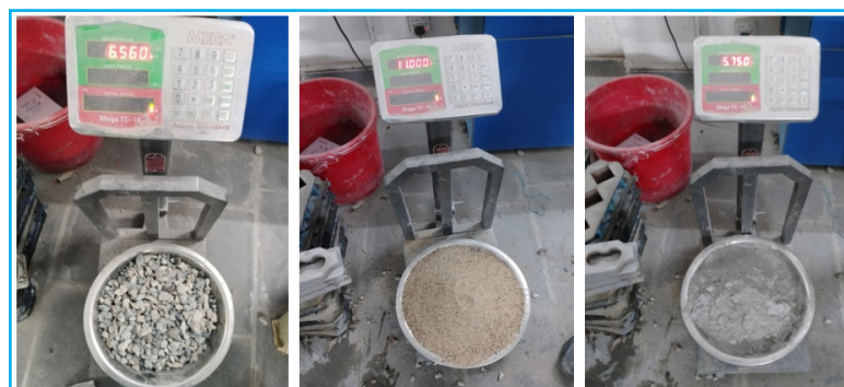
Figure 5. Weight based batching of aggregate, sand and cement
