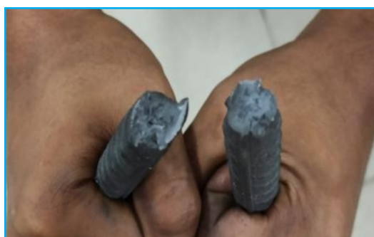
Figure 12. Failure of 20 mm of 40 grade rebar
