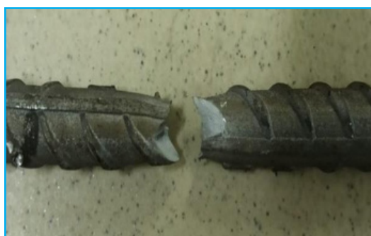
Figure 11. Necking of 20 mm of 40 grade rebar
