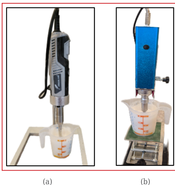
Figure 7. Mixing PEEK additive with mixing potable water (a) Mixing PEEK additive with mixing potable water using a mechanical homogenizer (b) Mixing PEEK additive with mixing potable water using an ultrasonic homogenizer
