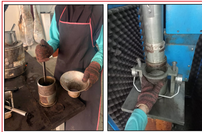
Figure 7. Marshall specimen preparation prior to testing, including mold filling, air void removal, and standard compaction
