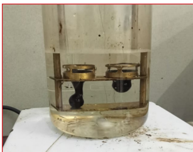
Figure 13. Ball 1 reached the softening point and dropped, while Ball 2 was approaching it
