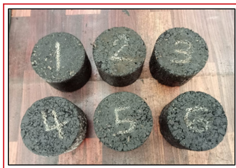
Figure 9. Marshall specimens after compaction, ready for testing
