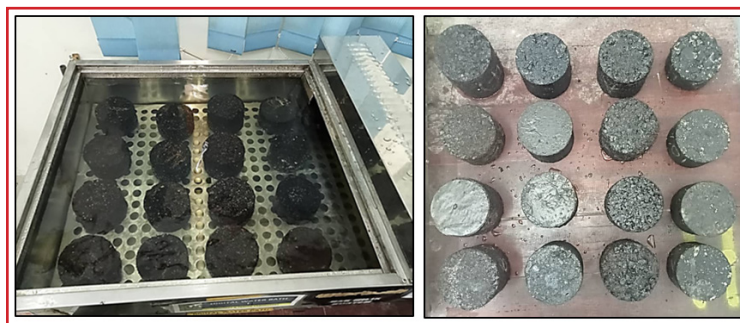
Figure 8. Marshall specimens during, and after water bath conditioning
