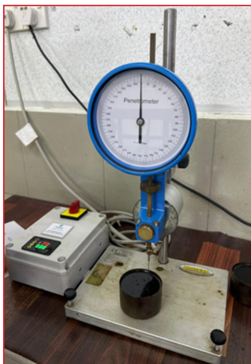
Figure 14. Penetration test apparatus during testing
