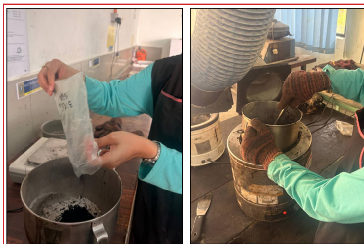
Figure 6. Incorporation of sugarcane bagasse ash (SBA) into the asphalt mixture through manual mixing to ensure homogeneity
