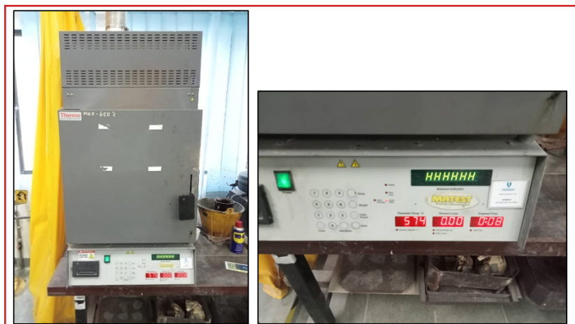
Figure 3. Combustion process of sugarcane bagasse in furnace
