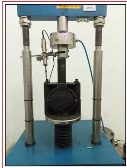
Figure 10. Marshall stability testing of asphalt mixture containing Sugarcane Bagasse Ash
