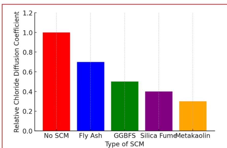
**Figure 3.** Effect of SCMs on chloride diffusion resistance
