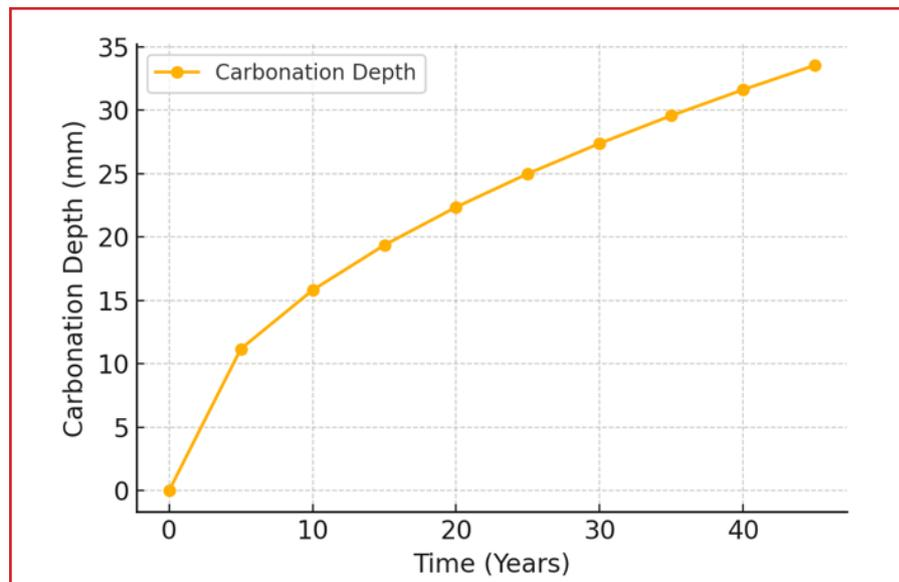
**Figure 1.** Carbonation depth over time in reinforced concrete
