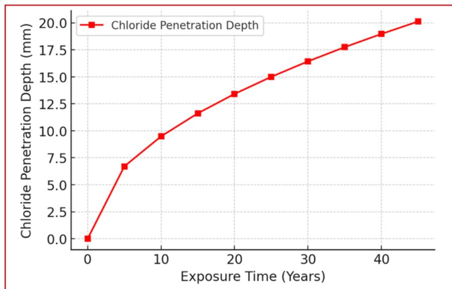
**Figure 2.** Chloride penetration depth over time in reinforced concrete
